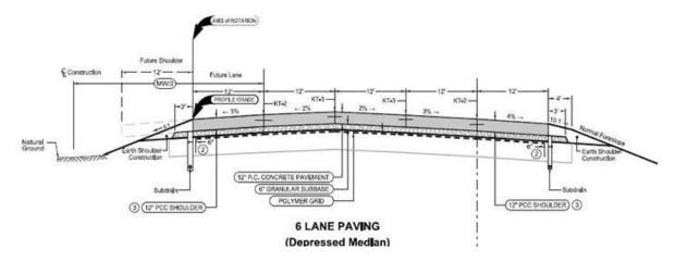
Figure 1: Detail showing polymer grid placement.
